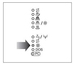
If the indicator light \* "Add rinse aid" on the control panel comes on, the <u>rinse aid</u> reservoir must be refilled.
